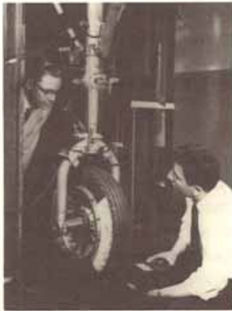
Investigations of the dynamic stresses that aircraft landing gear are subjected to were conducted for the growing aircraft industry in 1952. A significant increase in sponsored research characterized this period of the Department's history.
