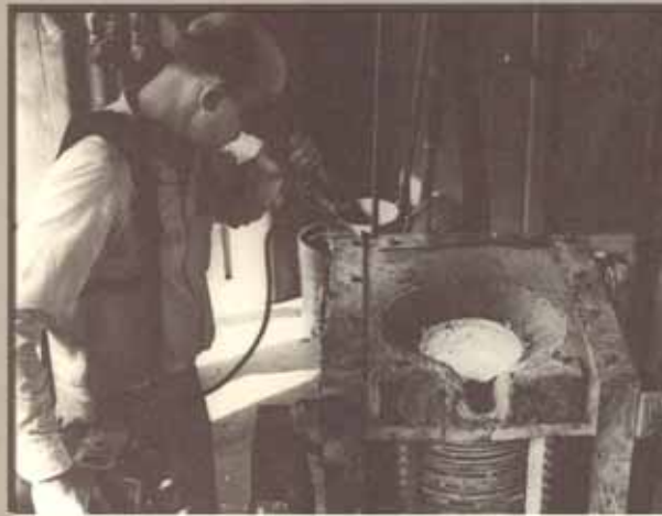
This optical pyrometer (ca. 1954) enabled a production engineering researcher to measure temperature in this induction furnace. The device utilized the human eye to compare a heating element to visible, radiating color. Before the advances in electronic imaging technology of the 1980s, many devices tried to assist natural vision in making measurable observations.
