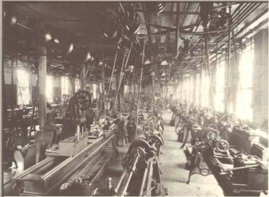
This machine shop, located in the second floor, was used for student work in blacksmithing and machine tool work. The building included its own power plant, and line shafts powered the belt-driven machines.
