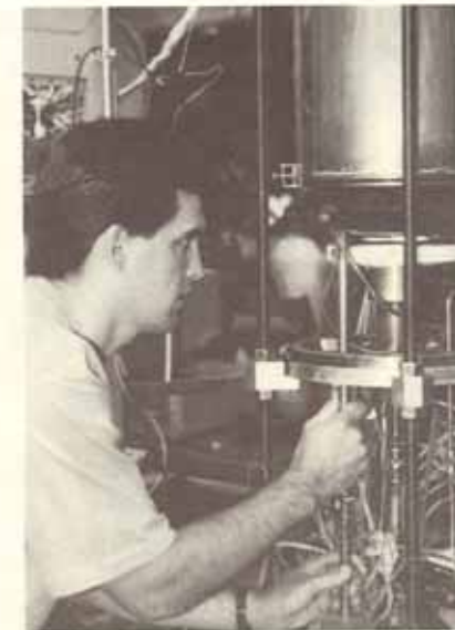
Researchers in Prof. Arvind Atreya's laboratory evaluate fire suppressants and the basic mechanisms of fire suppression using one-dimensional laminar diffusion flames produced in this stagnation point flow apparatus.
