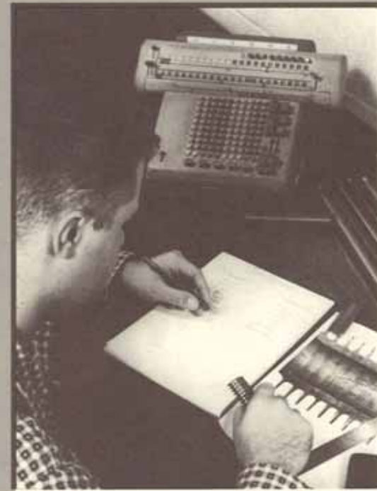
From slide rules to supercomputers, devices for scientific calculation have gone through amazing changes in the last 125 years. This researcher is using a Monroe Calculator in his examination of heat exchanger coils.
