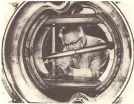
The Willow Run Laboratories provided research opportunities for studies in aerodynamics, engine research, and aviation electronics. This supersonic wind tunnel, capable of generating streams of up to 3,000 mph., was used to study fluid flow and heat transfer behavior of sudden pressure shock waves and the flow of gases behind them. Such studies enabled researchers to explore the effects that breaking the "sound barrier" would have on vehicle design.
