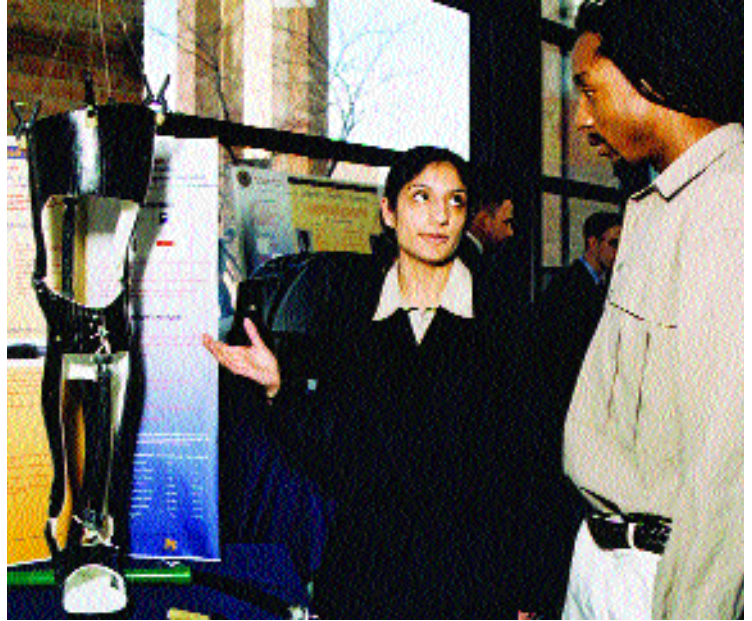
This pneumatic hip-knee-ankle-foot orthosis is designed to assist in gait rehabilitation. The team's goal was to "minimize the weight and size of the brace, optimize the location of the four muscles on each leg, maximize the joint range of motion and size of the muscles, design a system that mimics the patella, and simplify the use of the orthosis."
