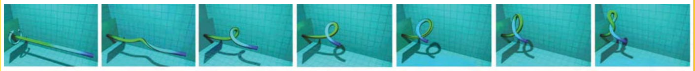
Results from early collaboration with Lawrence Livermore National Laboratories illustrating the evolution of an interwound supercoil (a plectoneme) under slowly increasing twist applied at left end.
