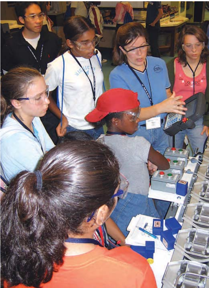
Professor Tilbury demonstrates how to program the robot from the teach pendant.
