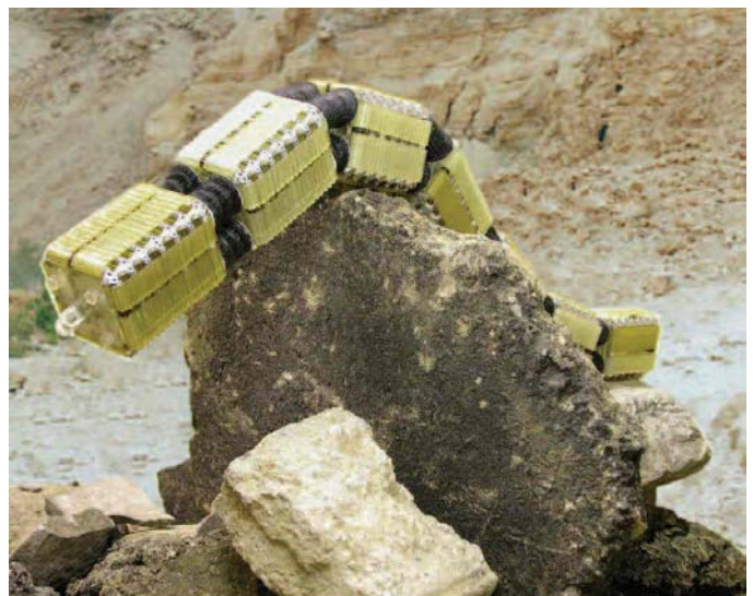
The OmniTread serpentine robot is designed to traverse extremely difficult terrain, such as the rubble of a collapsed building. It can drive over sand and rocks, as well as pass through small holes and climb over tall obstacles.
