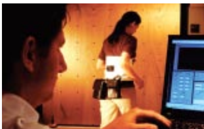
Sienko's balance prosthesis device consists of a motion-sensing system mounted on the lower back of the subject, a vibrotactile display and a laptop computer (or wearable watch) with analog and digital interfaces. Image courtesy of Draper Laboratory.
