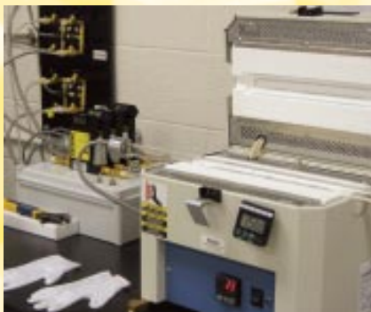
Atmospheric pressure tube furnace for nanotube and nanowire growth.
