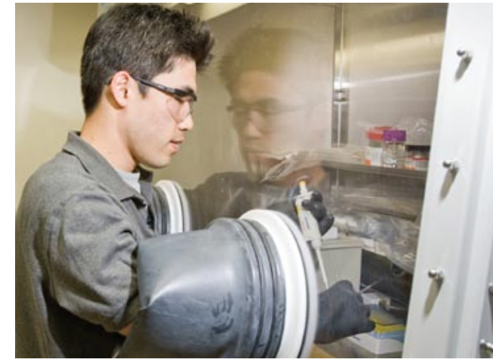
ABOVE: Dr. Myoungdo Chung prepares advanced battery materials for characterization and cycling. RIGHT: Fracture in particles in battery cell cathodes is being studied. The problem is challenging because of the complex architecture of the systems.
