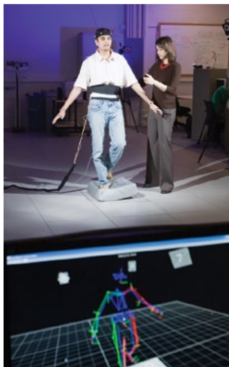
LEFT: Assistant Professor Kathleen Sienko, and graduate student Vivek Vichare evaluate a vibrotactile feedback device for improving balance.
