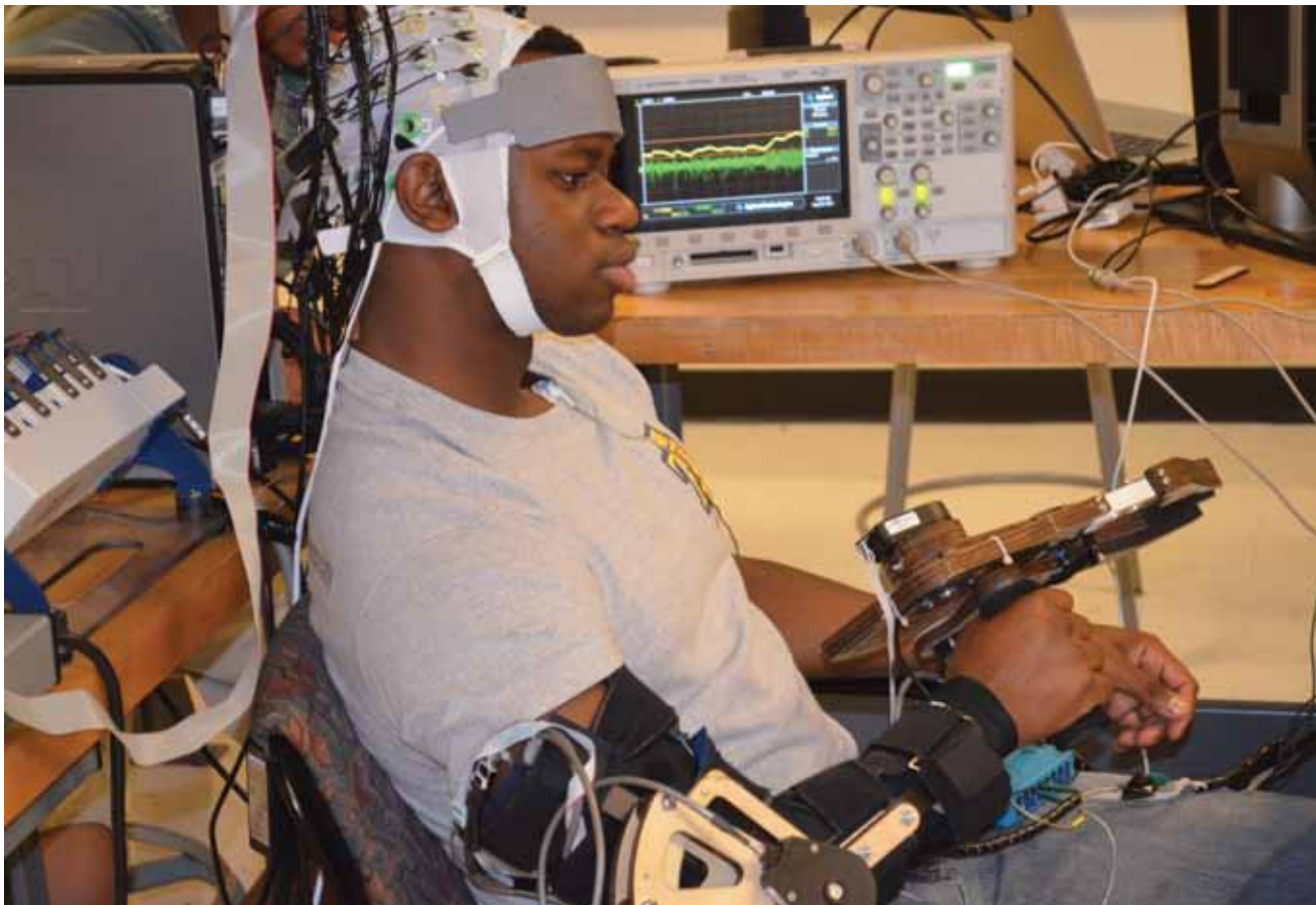
ABOVE: Encephalography and functional Near Red Spectroscopy are used to monitor the neural activity of Brandon Johnson, a member of the Haptix Lab, as he prepares to grasp and lift an object using a prototype smart prosthetic device. The instrumented terminal device that Brandon holds and motorized exoskeleton he wears about his elbow models the myoelectric control and sensory feedback being developed for use by upper limb amputees.
