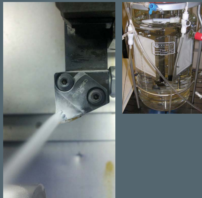
BOTTOM LEFT, RIGHT: Recycled carbon dioxide spray removing heat and delivering controlled quantities of lubricant to a machining process
