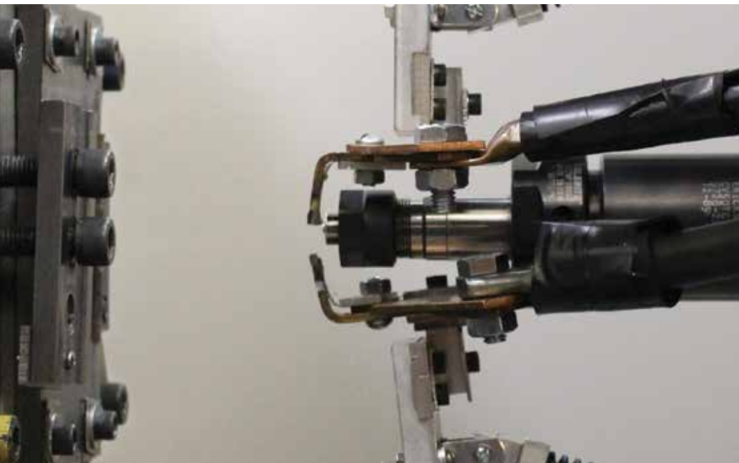
RIGHT: FSW welded specimen of Aluminum alloy Al6061 joined with advanced high strength steel: TRIP steel.
