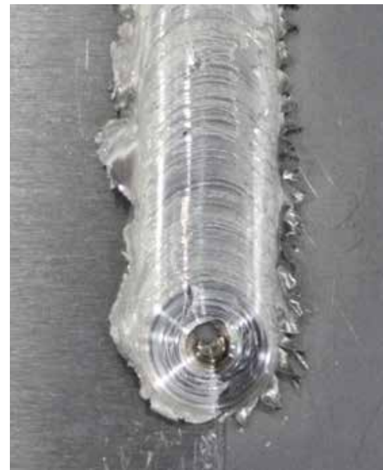
RIGHT: FSW welded specimen of Aluminum alloy Al6061 joined with advanced high strength steel: TRIP steel.
