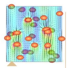
Professor **Grétar Tryggvason** researches direct numerical simulations of multiphase bubbly flows, which occur in both industrial and natural processes. In this simulation, 27 deformed bubbles are rising with an average rise Reynolds number of 20.
