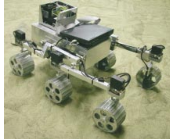
FLEXnav PPE (Proprioceptive Position Estimation) system is shown mounted on the Rocky-8B Mars Rover clone. The system is under development by Senior Research Scientist Johann Borenstein and Research Investigator Lauro Ojeda.
