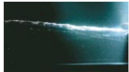
Cavitating vortices interact in the wake of two hydrofoils mounted in the U-M nine-inch water tunnel.
