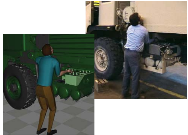
Human simulation, such as modeling the effort required to replace heavy duty truck batteries, allows manufacturers to evaluate the maintenance requirements of future vehicles and propose re-designs of current vehicles.
