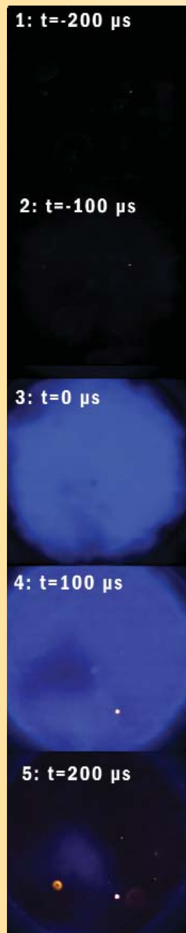
Typical ignition sequence for \phi = 0.4 , 10,000 fps, 90 \mu\text{s} exposure.
