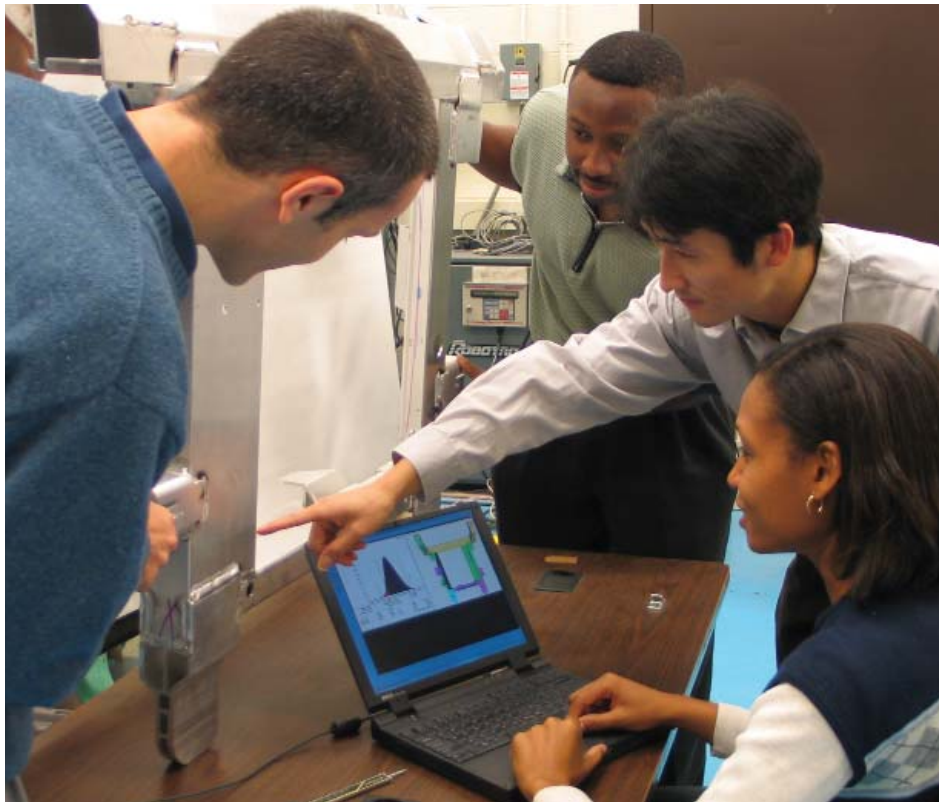
Graduate students Eduardo Izquierdo, April Bryan, Jianpeng Yue, Chino Imediegwu compare results of variation simulation models with actual measurements in order to determine the areas of highest variation of an aluminum engine cradle.
