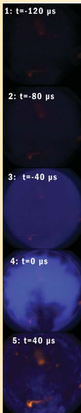
Typical ignition sequence for \phi = 0.6 , 25,000 fps, 19 \mu\text{s} exposure.
