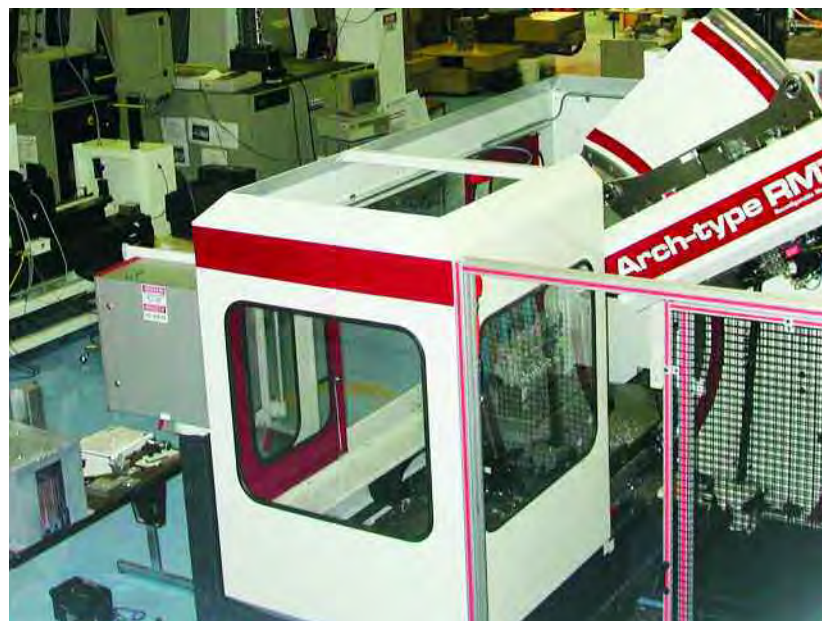
The ERC-RMS "Arch-type" reconfigurable machine tool (RMT) is the first of a new generation of easily reconfigurable production machines. It was built for the Center by Masco Machine Tool in 2002. The Arch-type is able to perform as a horizontal milling center as well as diagonal in 15° intervals.
