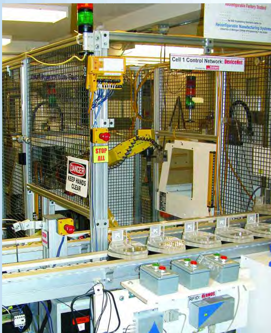
Students in Italy watch the ERC-RMS' Reconfigurable Factory Testbed in Ann Arbor. Robot loaders (yellow) pick parts from a track and place them into machine tools (white aperture) for processing. The testbed allows for the integration of a suite of machine operations, including real and virtual tools, as well as facilities in other factories. It can be controlled remotely via a Web-based human/machine interface.
