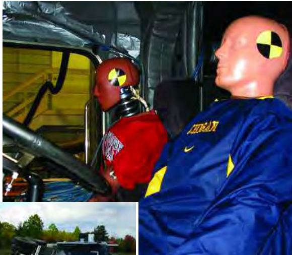
Making trucks roll over to validate computer models.
