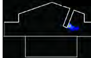
Images showing flame progress in the combustion chamber of an alcohol-fueled spray-guided spark-ignition direct-injection.
