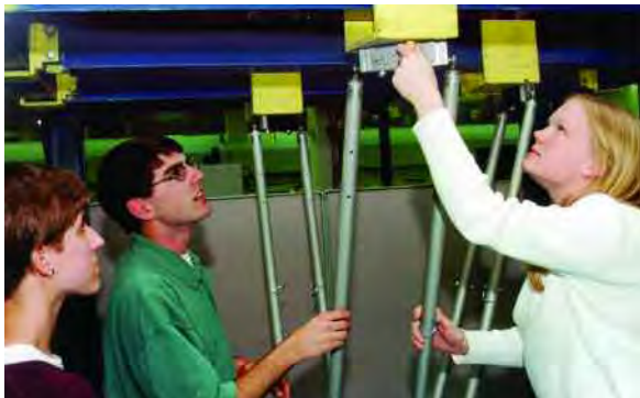
ME450 students working on a prototype parallel kinematic device in the ERC-RMS. The device works by sliding rigid elements closer to and farther from each other along parallel rails. The result is rapid, repeatable movement of a carriage connected at the bottom to all three elements.
